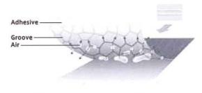
Air trapped between the BELBIEN and the substrate exits through specially designed narrow grooves as pressure is applied with the squeegee.
